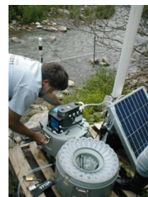
Fig. 3b. Servicing “R 2 D 2 ” the Teledyne ISCO automated water sampler located at the Rt 38A site. It
